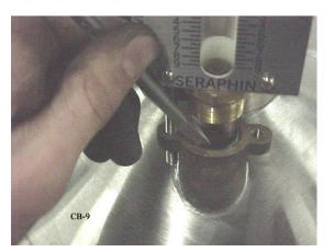
NOTE: Pictures shown are of a Test Measure. Although parts may vary slightly the same process can be used for Provers of all sizes. For larger Provers the seal must be broken and locking pin must be removed resulting in the need for recalibration.
