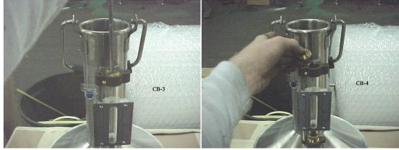
3. Using a 1" open end wrench (CB-5), unscrew the brass compression hex nut at the bottom of the gauge assembly.
