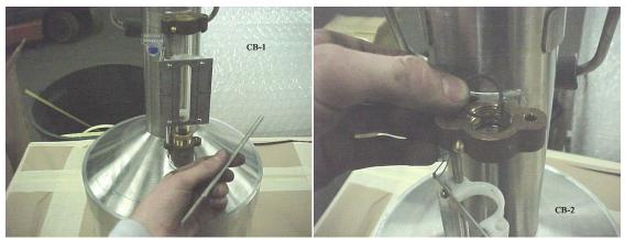
2. Remove brass plug (CB-3) for upper fitting with screwdriver (CB-4).
