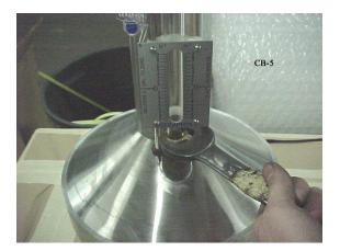
4. Carefully grasp the gauge glass (CB-6), lift and twist at the same time to remove from the gauge supports. Be sure to find the two "O" rings (CB-7) under the brass compression hex nut, as they do not always come out with the glass (CB-8).
