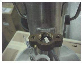
5. To re-install reverse the process, carefully putting the "O" rings around the tube where necessary (CB-9). Tighten the compression nut so that you cannot twist the gauge glass in the assembly.
